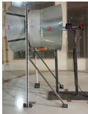
Figure 1. DHAWT model installed in the wind tunnel test bench, lateral view, 1) concentrating duct, 2) diffuser 3) torque-meter Interface T25 4) magnetic powder brake.
